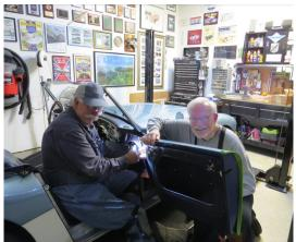
back plate to use as locating holes with 1/8" drill bits during assembly. That tip was invaluable - it was also used the same way before removing the hood and the locating holes provided prefect hood alignment. With the
